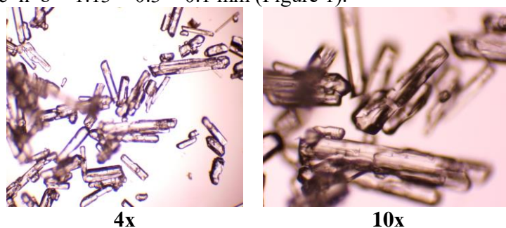
Figure 1. Micrographs of Potassium nitrate crystals ( \times 4 and \times 10 ) obtained from the samples prepared according to Table 1
