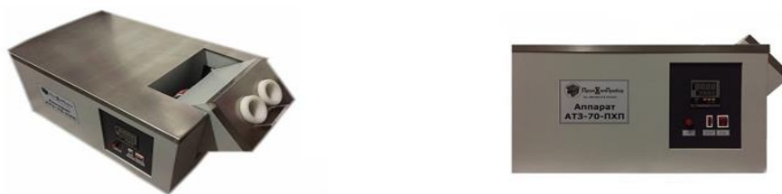
Figure 1. ATZ-70-PXP freezing temperature detector
